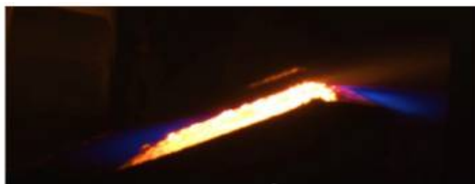
Figure 1: ESIMOUN (arc-jet heater) wedge specimen for the tile pattern and aerothermal instrumentation qualification campaign
