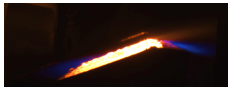
Figure 2: SIMOUN (arc-jet heater) wedge specimen for the tile pattern and aerothermal instrumentation qualification campaign
