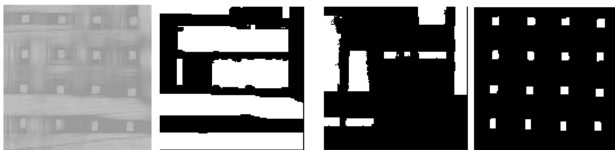
Figure 1: Sample tow segmentations using the method based on SAM's automatic mask generation. Images from left to right are original CT scan, X-tow, Y-tow, and Z-tow segmentations, respectively.
