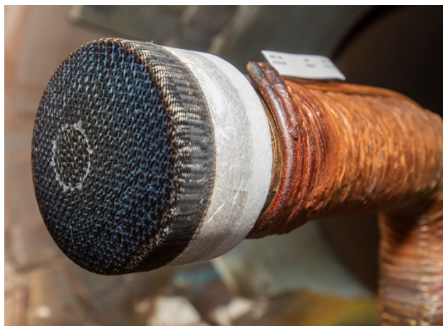
Figure 1: A 4-inch iso-q model made from 3MDCP tested in the IHF arcjet.
