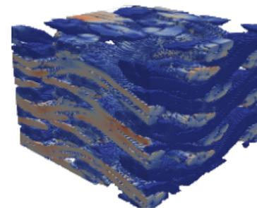
**PATO used to analyze mechanical properties of woven TPS material for MSR-EES using micro-CT data**
