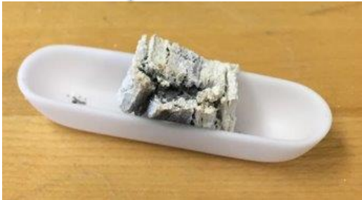
High temperature : dense oxide layer
