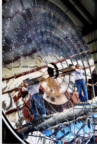
Solar testing (solar furnace, chamber, and plasma facility [Anderson]) – 600 \text{ W/cm}^2 , 3000 \text{ C}
