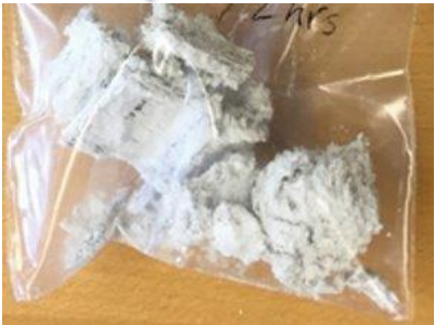
Medium temperature : powdered oxide layer
