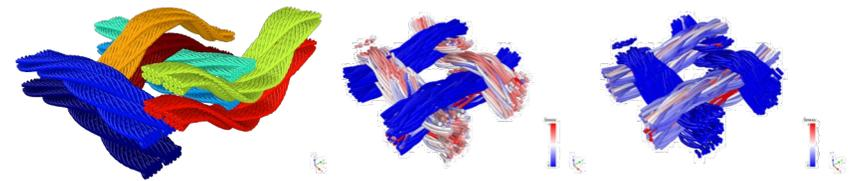
LAMMPS and HYDRA employed to study mechanical-mediated failure of weaves and the damage and propagation resulting from ballistic testing impacts
