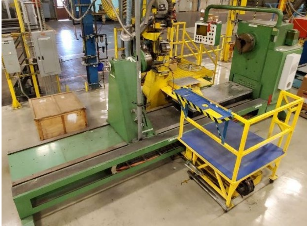
Tape winding of TPS materials
