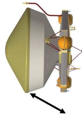
PICA "tooth" design being traded for Dragonfly heatshield to provide protection of main seal – performance assessment requires multi-D capability
