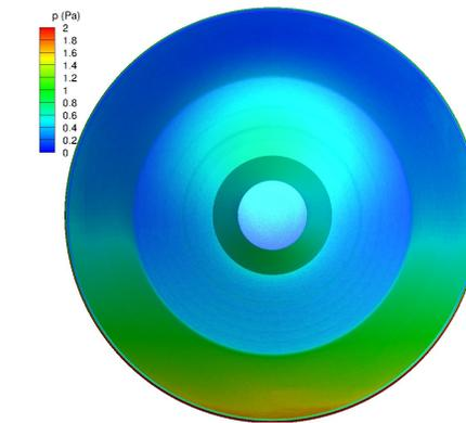
**SPARTA used for accurate characterization of Mars2020 backshell and shear stress on woven TPS for MSR-EES to inform spallation**
