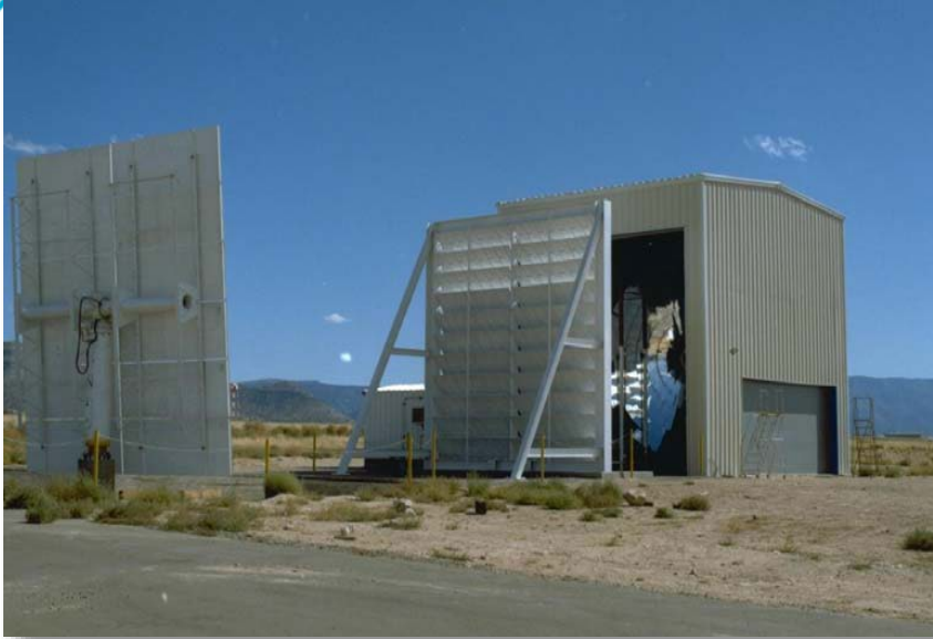
Solar testing (solar furnace, chamber, and plasma facility [Anderson]) – 600 \text{ W/cm}^2 , 3000 \text{ C}
