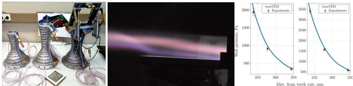
Figure 1: Three new supersonic nozzles commissioned at VKI (left); flat plate copper calorimeter test with semi-elliptical nozzle (middle); comparison of pressure distribution along divergent nozzle part for two conditions to simulations (right).
