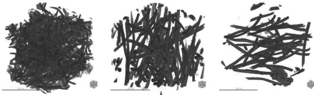
Figure 2: Virgin Carbon Felt with UHT (left), Charred Normal Carbon Felt with UHT (center), Charred Purified Carbon Felt with UHT (right)
