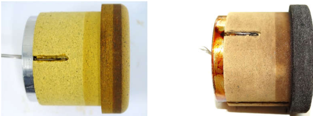
Figure 1: Density graded ZURAM sample before and after test in arc-heated wind tunnel facility L2K (DLR, Cologne).
