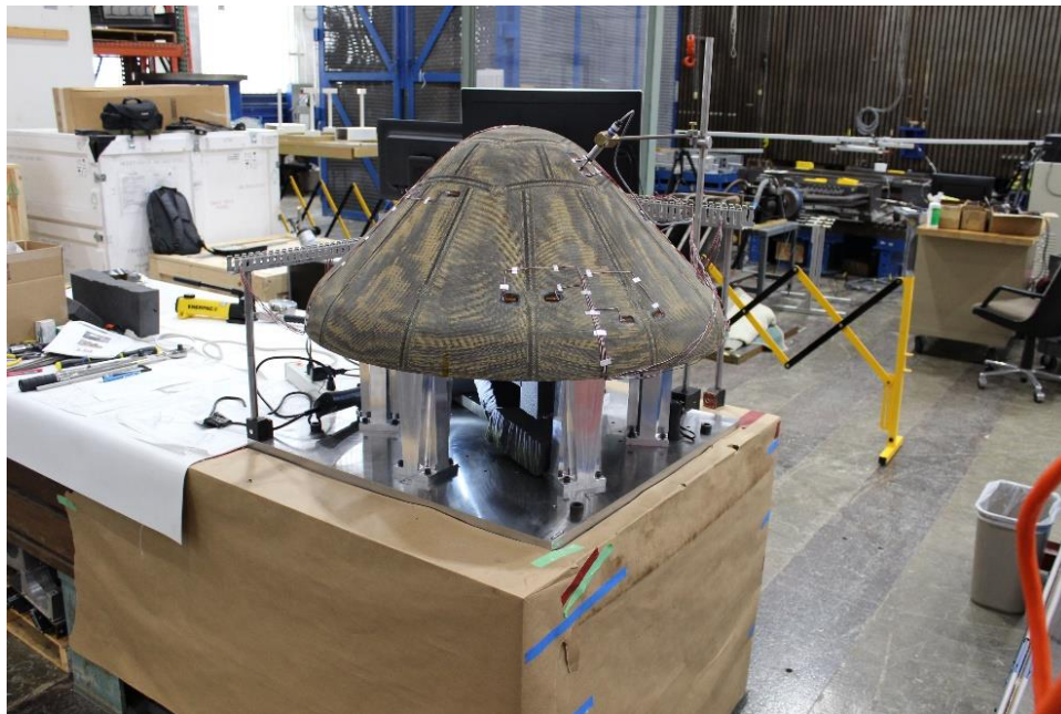
Figure 1: ETU Static Point Load Test Setup
