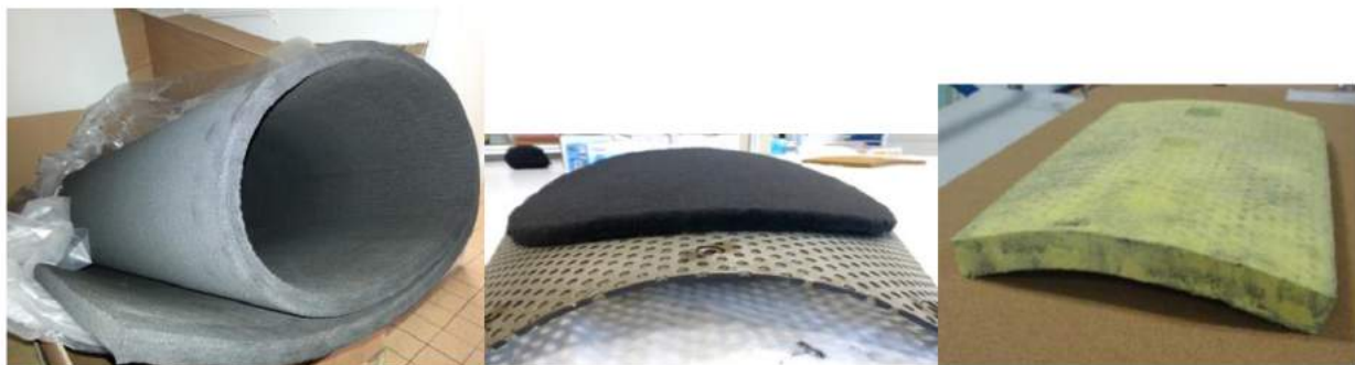
Figure 1: As received flexible felt, Conformal ASTERM before and after impregnation (from left to right)
