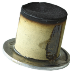
Figure 1: Sample of ZURAM R after 15 sec at 12 \text{ MW/m}^2 at PWK1 (IRS, University of Stuttgart)
