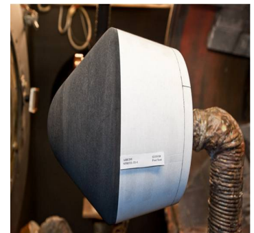
Figure 3: SPRITE model after exposure to plasma flow
